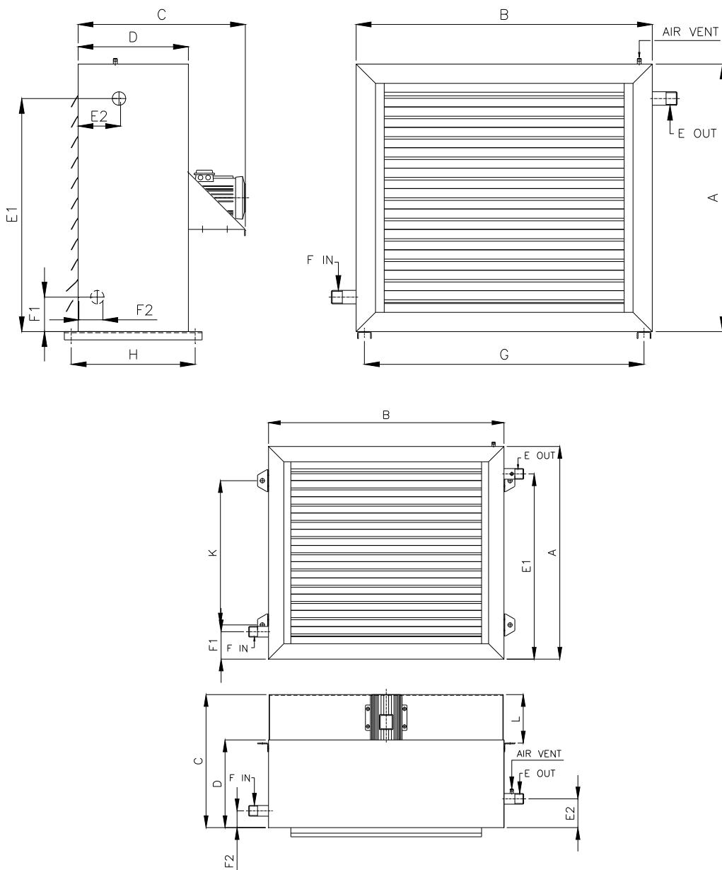
FIGURE 3. HIGH CAPACITY HOT WATER UNIT HEATER
