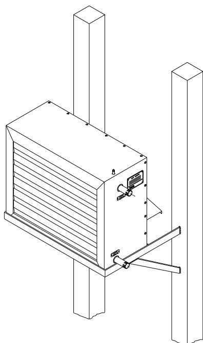
FIGURE 7. MOUNTING TO COLUMNS
